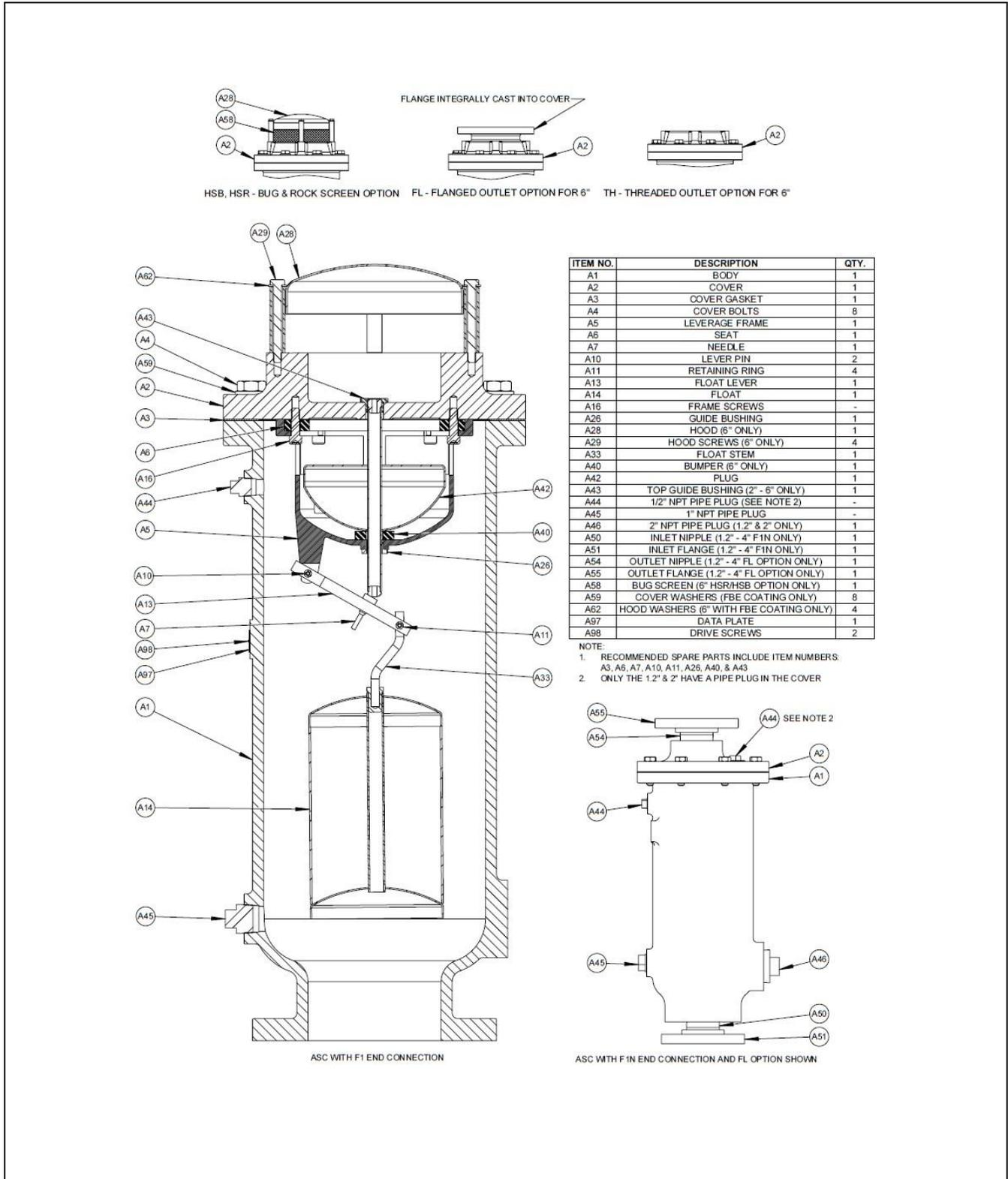
Figure 1: ASC Single Body Sewage Combination Valve
