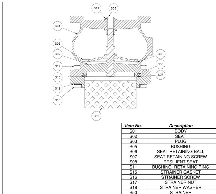
Figure 1: APCO FFF-1400A Full Flow Foot Valve
