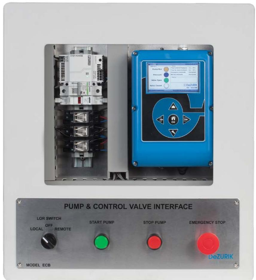
provides visual indication of system status. The colored lights indicate normal operation and alarm conditions of the pump and control valve. Pump run/off, pressure switch and valve open/closed status are displayed with colored indicator lights. The Time for System to Build Pressure and the Time for Valve to Open are displayed as time in seconds, while on solenoid controlled valves the emergency and normal solenoid status indicates if the solenoid valves are energized or de-energized.
