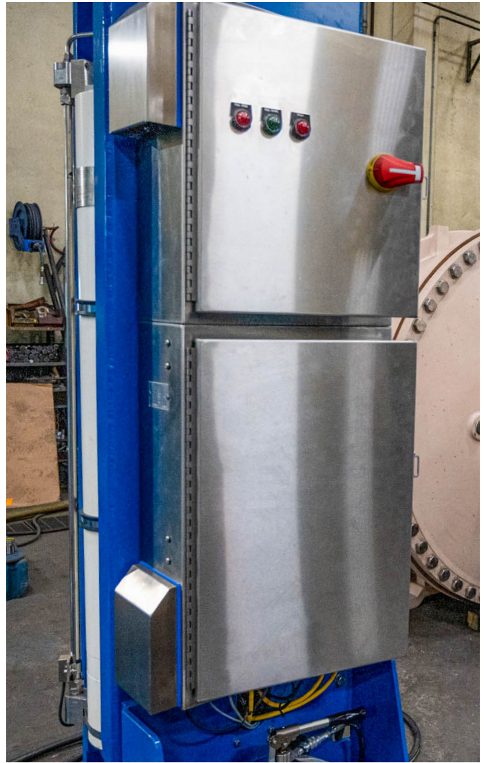
The DeZURIK HPUs were custom engineered to have a specified footprint.
