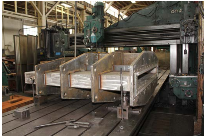
In-house machining, 72" Bonneted Knife Gate Valve
