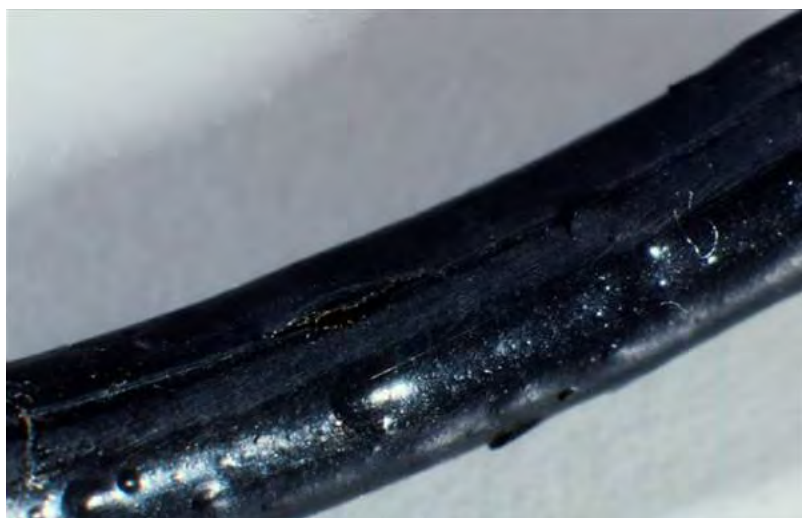
Figure 2. An example of a fluoroelastomer seal that has swollen as a result of an amine chemical attack (source: Gallagher Seals). 10
