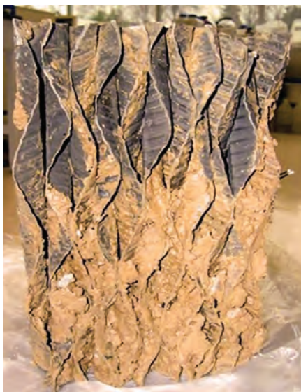
FIG. 3. Fouled cooling tower film fill.
