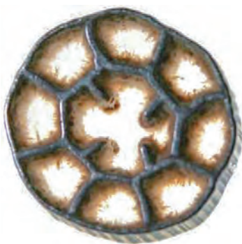
FIG. 7. Attached growth on MBBR media surfaces.
