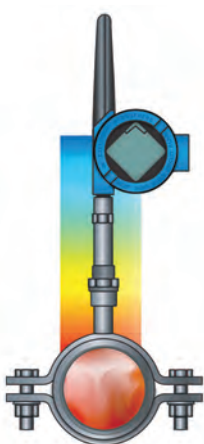
FIG. 10. Where it is not practical to add a permanent temperature measurement point, a transmitter h can infer the water temperature without a process penetration.
