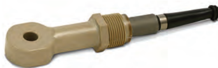
FIG. 6. Where suspended solids levels are high, a toroidal conductivity sensor d may be necessary to make the measurements used to reduce the level.
