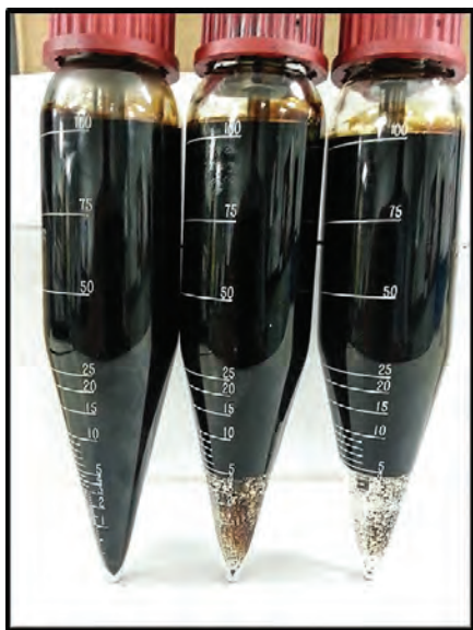
FIG. 5. Tubes containing crude and demulsifying chemical for PED tests. Photo courtesy of Dorf Ketal, USA.
