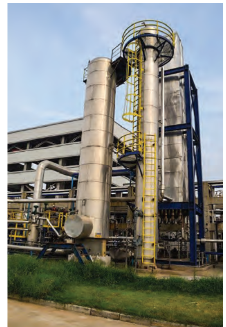
FIG. 2. The refinery's WAR is used to reactivate spent powdered activated carbon from its PACT system.
