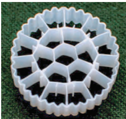
FIG. 2. This proprietary MBBR carrier reduced influent distillable phenols to 40 µg/L–48 µg/L, while benzene could be detected only in the third sample, with a reduction to 24 µg/L in samples from a refinery wastewater treatment plant in Sweden.
