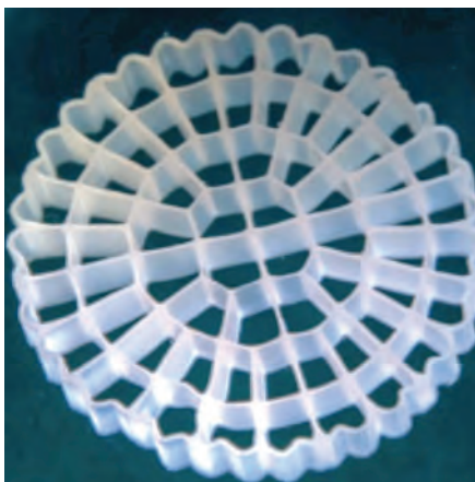
FIG. 3. This proprietary MBBR carrier reduced phenols to 19 µg/L–79 µg/L. Benzene removal was below the detection limit of 0.5 µg/L on all samples collected from the effluent of the second reactor. Measured benzene concentration was above the detection limit twice in a laboratory test.
