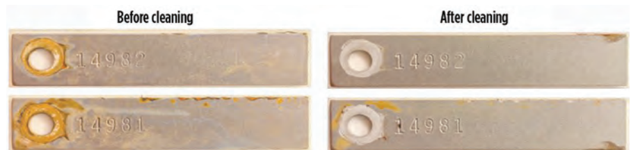
FIG. 8. Mild-steel coupons placed at the hot exit temperature of heat exchangers. The average corrosion rate was 0.25 mpy, one-tenth of industry corrosion standards.
