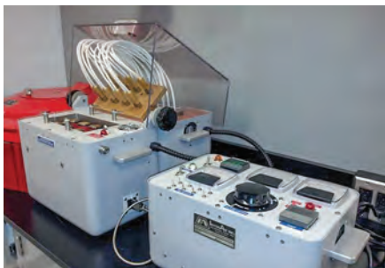
FIG. 4. Portable electric desalter in a laboratory. Photo courtesy of Dorf Ketal, USA.
