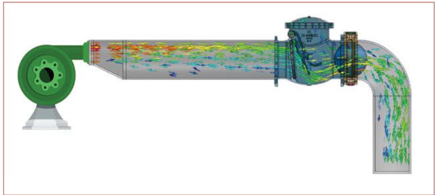
Moving the check valve further from the increaser decreased turbulence and allowed flow to become more laminar.
